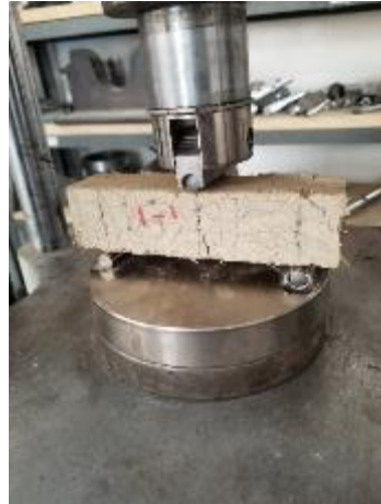
Figure 22. Schematic of flexure rupture test.
