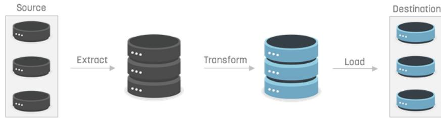
Figure 3. Example of an ETL Process
