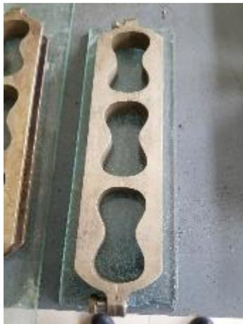
Figure 12. Mold for tensile test
