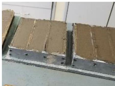
Figure 21. Flexure test specimens
