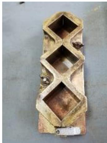
*Figure 10. Mold for compression test*
