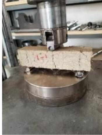
*Figure 22.* Schematic of flexure rupture test.
