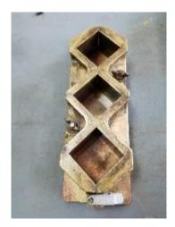
*Figure 10.* Mold for compression test *Note:* Source: Own elaboration, 2019
