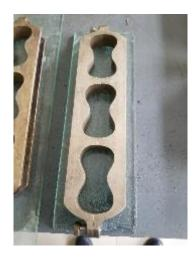
*Figure 12.* Mold for tensile test *Note:* Source: Own elaboration, 2019
