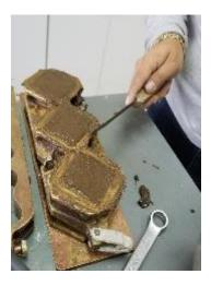
Figure 15. Compression test specimens
