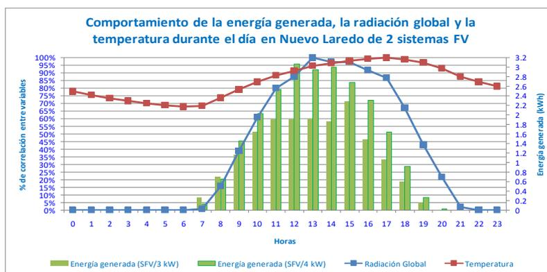
Figure 14. Comparison of meteorological variables and PV-generated energy.
