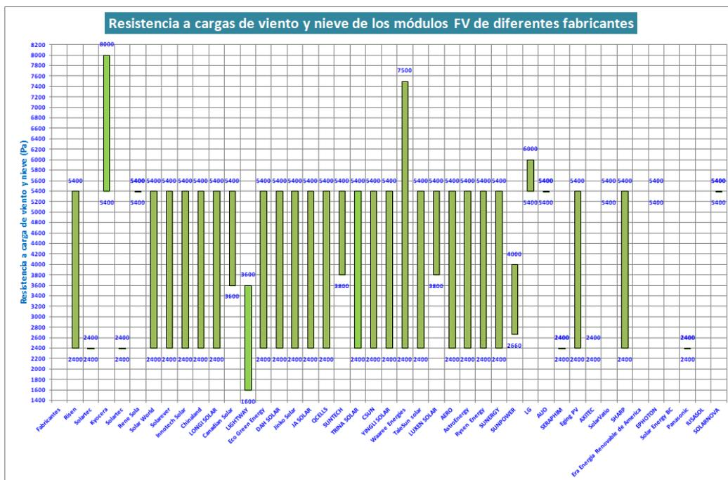
Figure 8. Resistance to mechanical loads of PVMs
