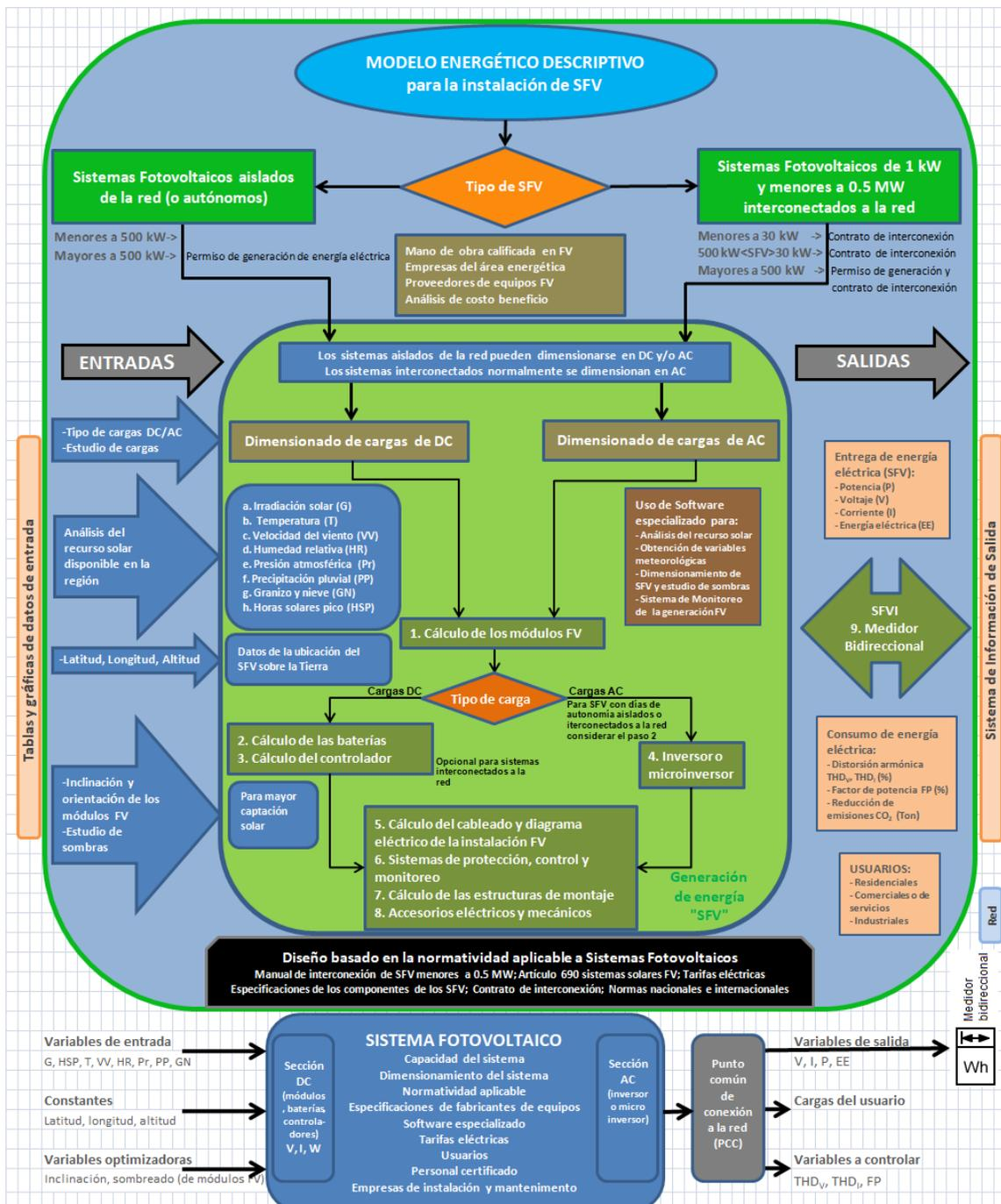
Descriptive model of a grid-connected solar photovoltaic energy system.
