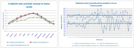
*Figure 3.* Solar irradiance and radiation measurements *Note:* Source: Own elaboration with data from RetScreen software, Meteonorm, and in situ measurements.
