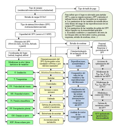
*Figure 2*. Flow diagram of a grid-connected PV energy system. *Note:* Source: Own elaboration.
