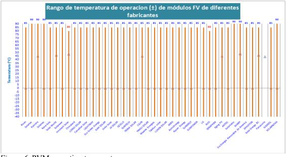
*Figure 6.* PVM operating temperature *Note:* Source: Own elaboration with data from manufacturer's data sheets.
