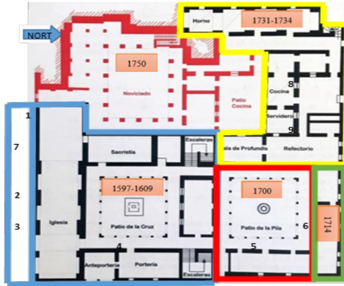
Figure 6. Delimitation of the construction periods of the San Diego Convent with the sample points
