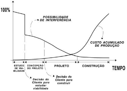
*Figure 3*. Relationship between the costs of the possibility of intervention and the accumulated production, through the phases of the construction project. *Note:* Source: Hammarlund and Josephson (1992), apud Melhado (1994).
