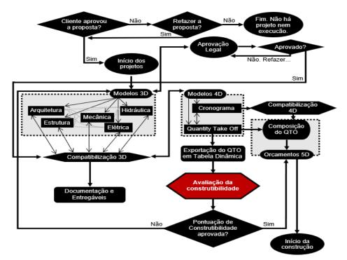
*Figure 4*. Constructability Assessment in an interdisciplinary BIM system *Note:* Source: by the author (2019).
