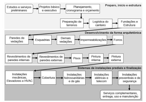
*Figure 2.* Process flow in the civil construction of buildings. *Note:* Source: by the author (2019), based on the empirical experience and recommendations of CBIC, as well as the management software manuals of "Work Breakdown Structure," WBS.
