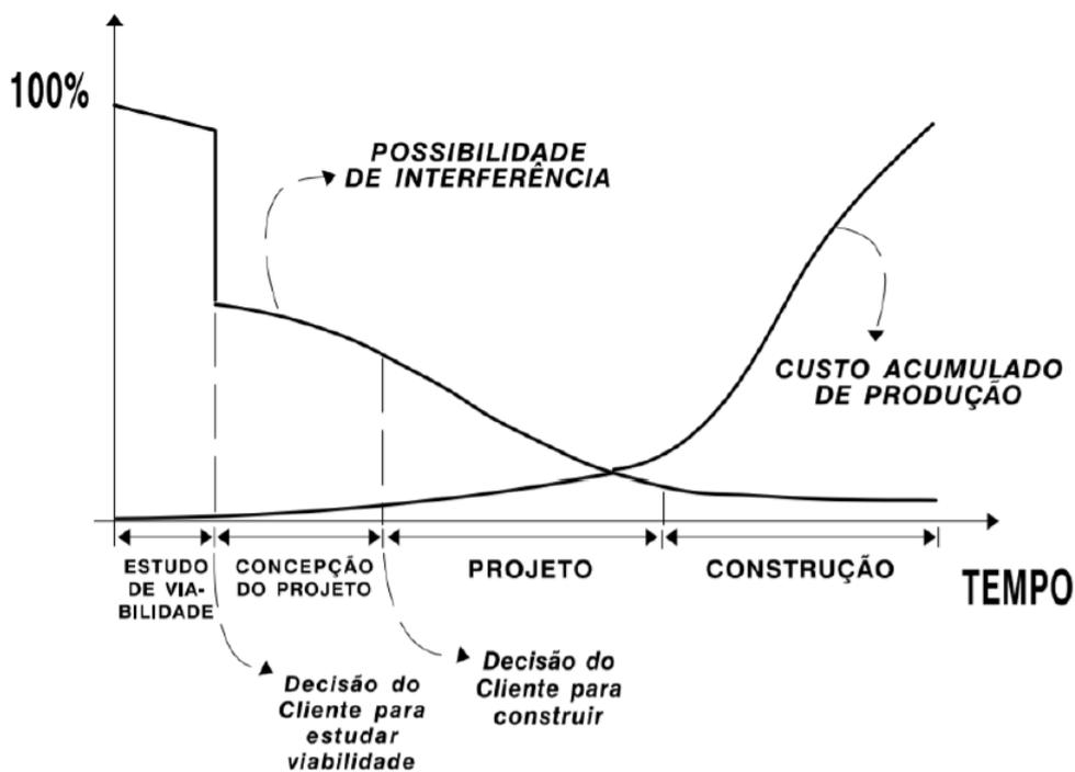
Figure 3. Relationship between the costs of the possibility of intervention and the accumulated production, through the phases of the construction project.
