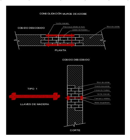
These keys were cured with *quimocide*<sup>11</sup>, to prevent them from being attacked by termites<sup>12</sup>, then they were painted with asphalt paint to protect these new timbers from the humidity absorbed by the walls and eliminated by condensation.
