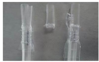
*Figure 21*. Acceptable weld, tube release test versus EVA or EVA/EVOH layer *Note:* Source: Author's creation.
