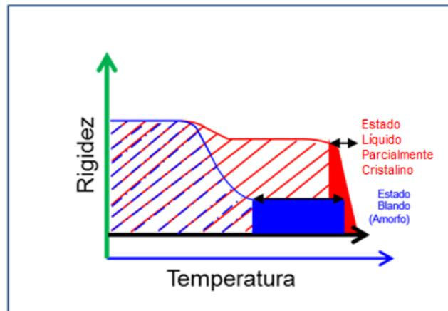
Figure 3. Graphic profile of semi-crystalline vs. amorphous materials.
