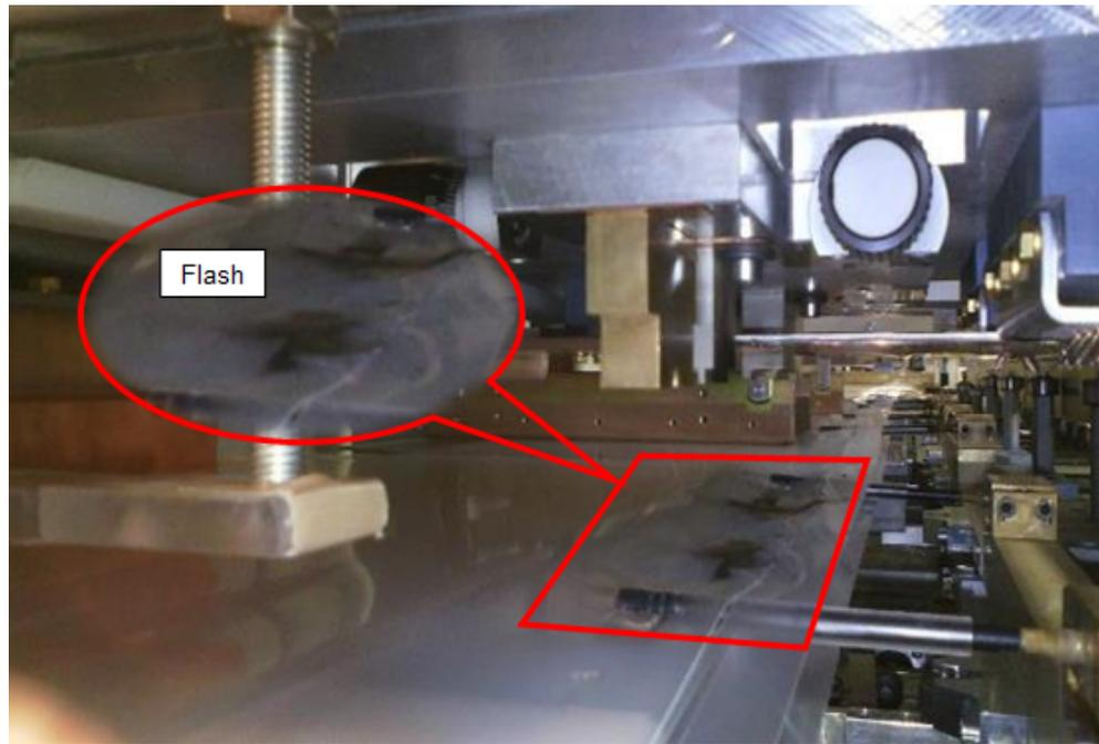
Figure 12. “Flash” effect on thickness specification welding
