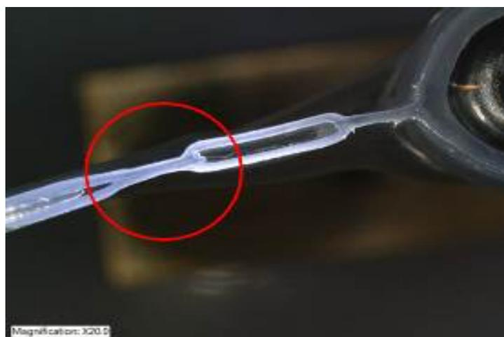
Figure 14. Material on weld with displaced material
