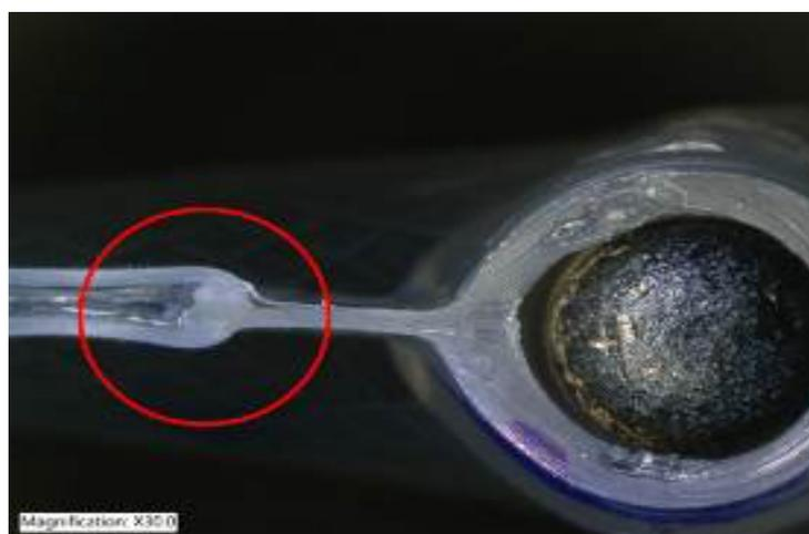
*Figure 16.* Welding rejected by visual inspection
