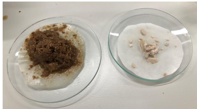
*Figure 3.* Cellulose (left) and hemicellulose (right) before drying.
