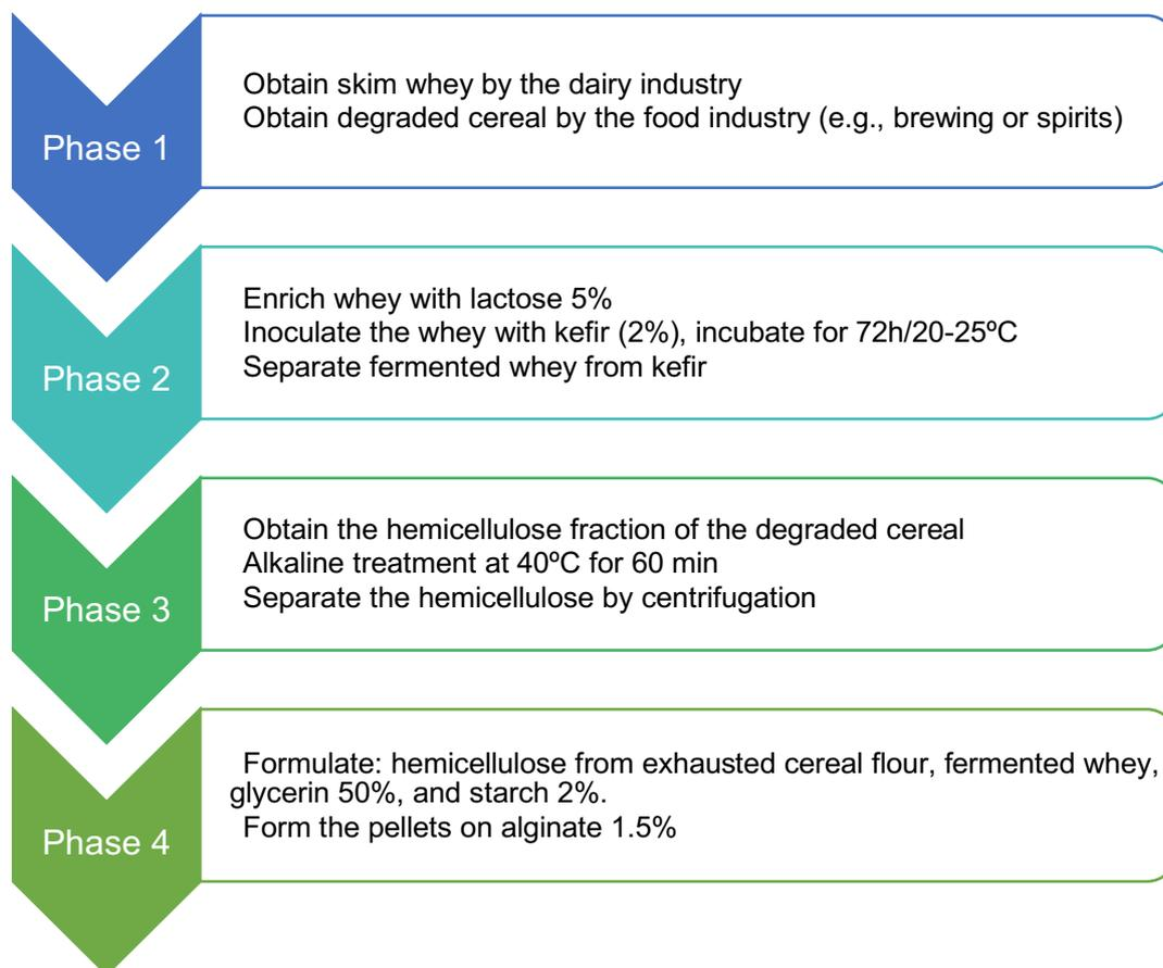
Figure 10. Bioplastic pellet production process
