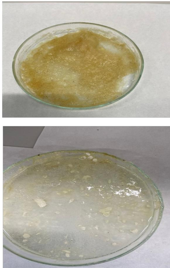
Figure 7. Comparison of the control biofilm (upper) with that of formulation 1 (lower)
