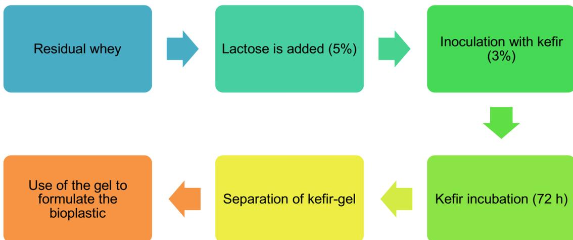
*Figure 4.* Process for obtaining biofilm gel at laboratory scale.
