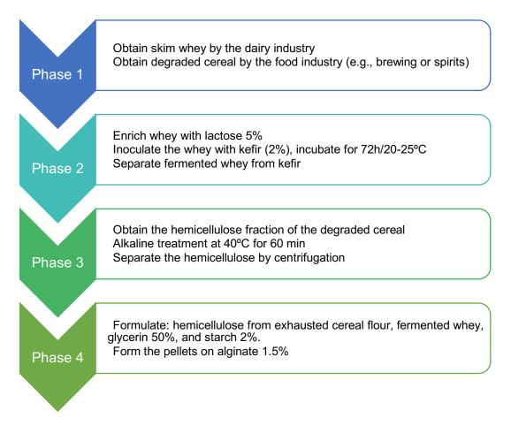
*Figure 10.* Bioplastic pellet production process *Note:* Source: Own elaboration, 2022
