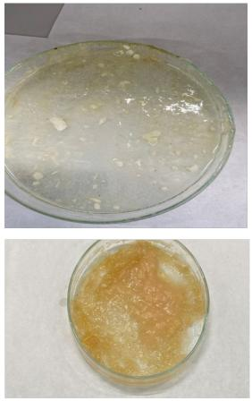
*Figure 8*. Comparison of formulation 1 (top) with the same formulation supplemented with 2% starch (bottom)
