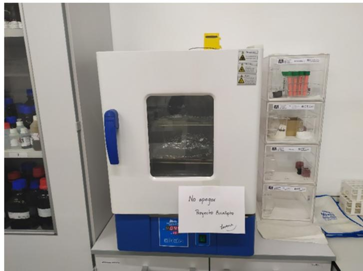
*Figure 6.* Oven-dried samples subjected to the drying process
